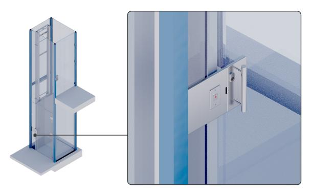
3a. When there are glass sidelights, door and sidelight housings are used to hold the door hardware and call button, and to provide a path for the wires. The sidelight housing will be the full width of the sidelight and butt up to the SHS post or wall, as above.
