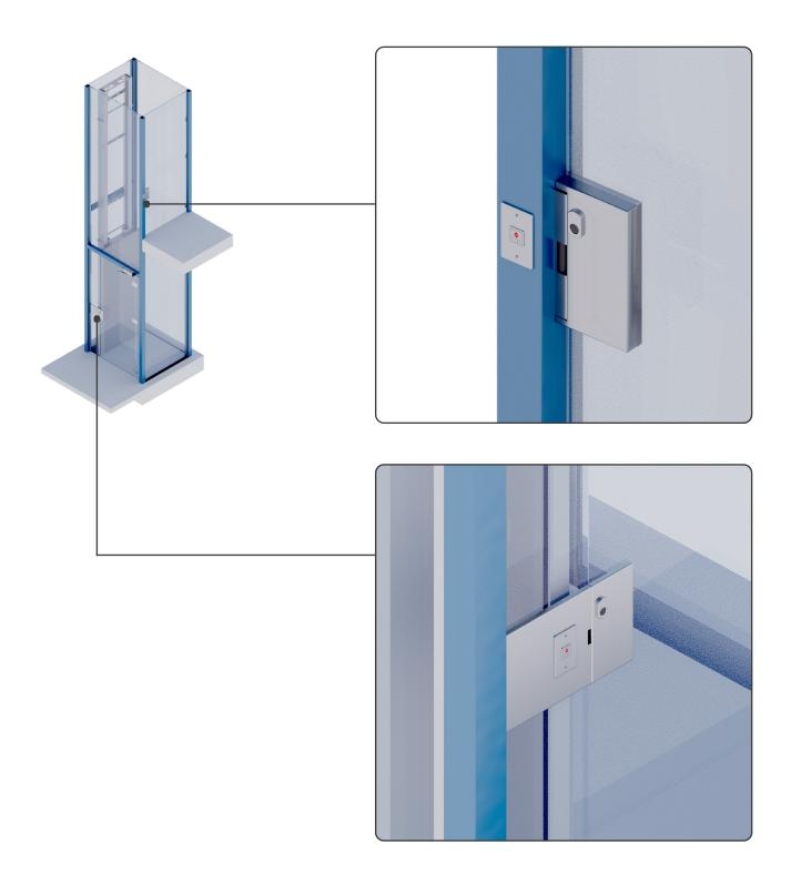
Call buttons are the same as in residential elevators, with all wiring going through the corner posts down into the pit and to the lift plant room.
