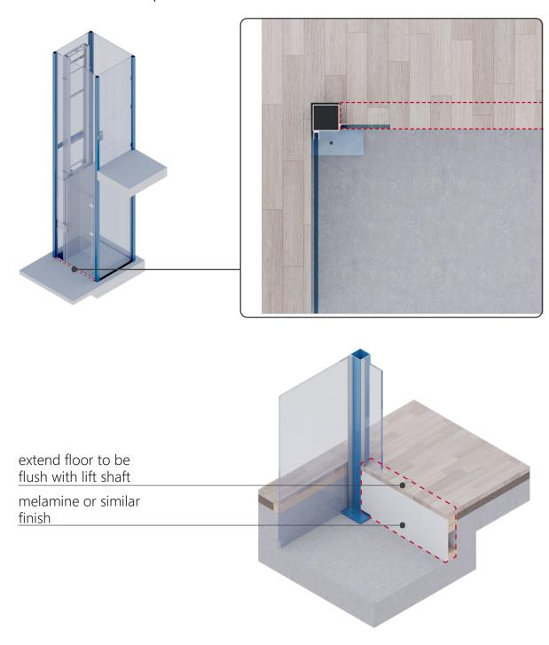
If the corner posts go into the pit as shown, a floor extension should be added to the pit wall on the door side which effectively brings the pit wall flush with the landing door, which is flush with the inside of the posts. Flooring can then be installed on top of the extension.
