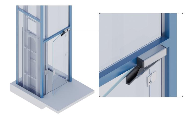
An SHS beam (or similar hollow section) is required to provide a mounting surface for an auto door opener.
