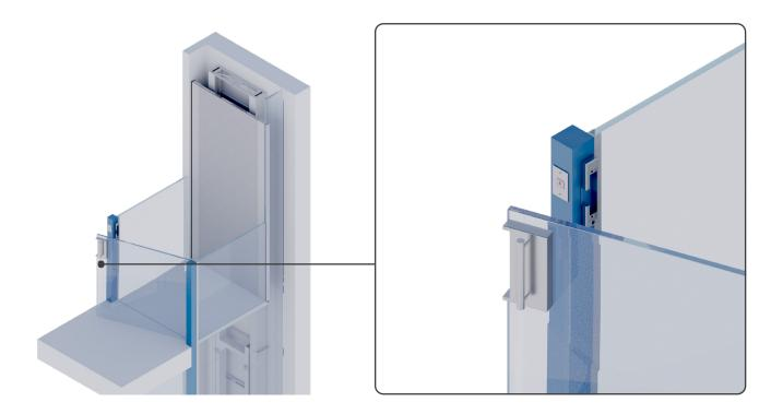
3d. When the doors are latching directly into a corner post, the lift call button is mounted on the corner post, the strike is mounted on the corner post, and a housing is used to mount the mortise latch in the door.
